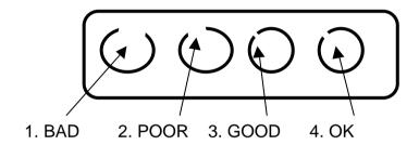
TECHNICIANS SHOULD ADJUST THE GAP ON CONNECTOR 1 & 2 Before fitting the drive
